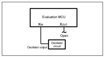
Figure 2.8 External oscillator circuit
